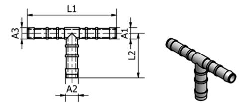
Ext. Hose Diameter A3 = 12 Ext. Hose Diameter A1 = 12 Ext. Hose Diameter A2 = 12 L1 = 69 L2 = 36
